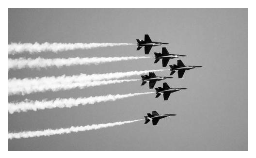
Condensed water vapor that comes from an airplane's engine makes cloudy streaks in the sky, called contrails.
